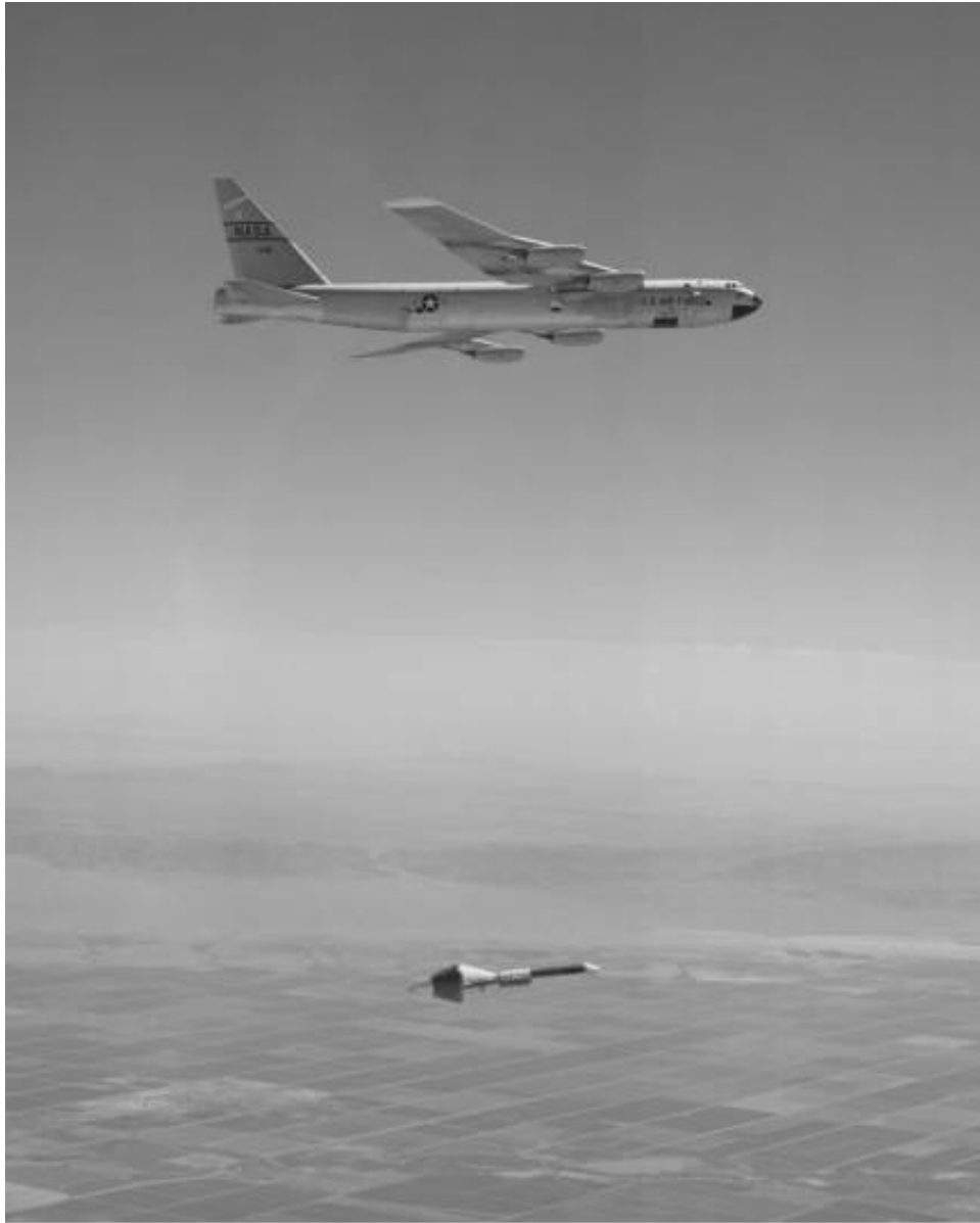
Figure No. E-8. Space Shuttle Solid Rocket Booster Drop Test Vehicle (SRB-DTV) first release from NB-52B, August 13, 1977.
